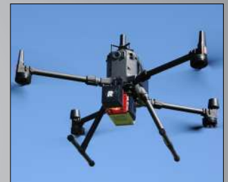
DJI Matrice M300 RTK equipped with RIEGL miniVUX-SYS using RIEGL Integration Kit 300
