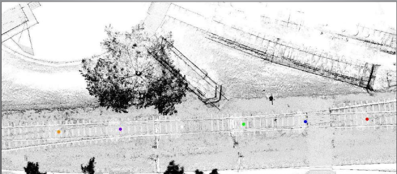
Pointcloud, orthogonal X-ray view from above: high level of detail on the track, the clearance and the surrounding area are included in the entire scan dataset.
