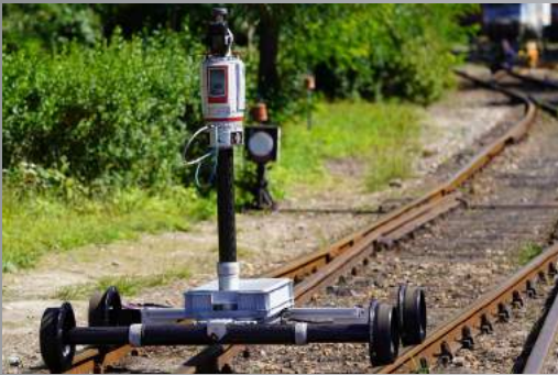
RIEGL VMR: data acquisition in Stop & Go mode at the test track in Lower Austria
