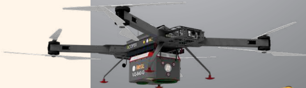
RIEGL VQ-840-G installed on RiCOPTER-M, RIEGL's remotely piloted aircraft system with exceptional payload capacity
